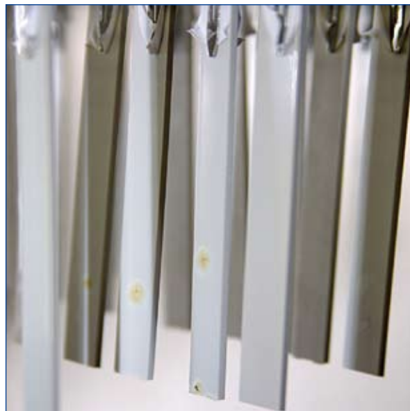
PP rods in the drying cabinet
